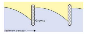
Groynes intercept the longshore movement of sand, and assist to retain sand on the beach between structures. Sand will accumulate to the side of the structure where sediment is moving towards. Some localised erosion can occur on the lee-side. Permeable groynes allow water to flow through at reduced velocities, while impermeable groynes block or deflect the current.
